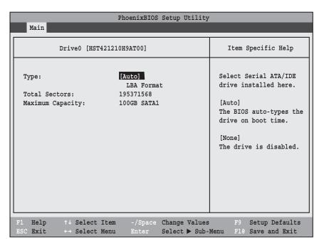
Figure 2. Drive0 Master Submenu
